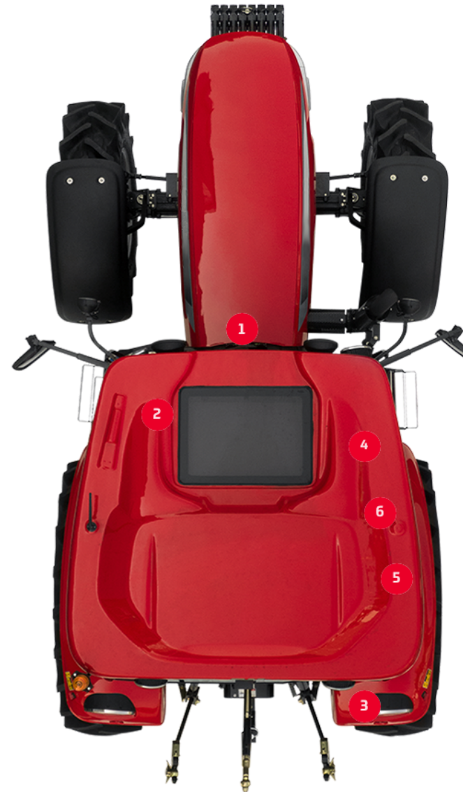
3. External button to adjust implement height
